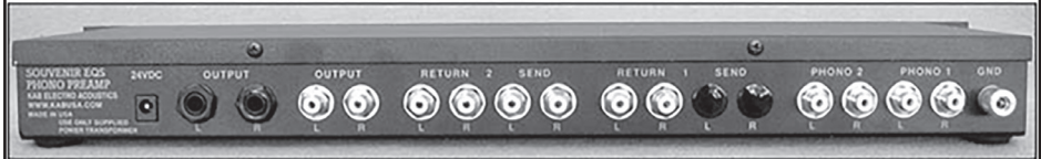
PHOTO 2: Rear panel of the EQS MK12. The ¼" jacks on the left are fully-balanced, tip-ring-sleeve outputs. RCA connectors are gold-plated and Teflon®-insulated. The jacks marked "Return 1" are actually the line inputs, which are placed ahead of the equalization circuits.
